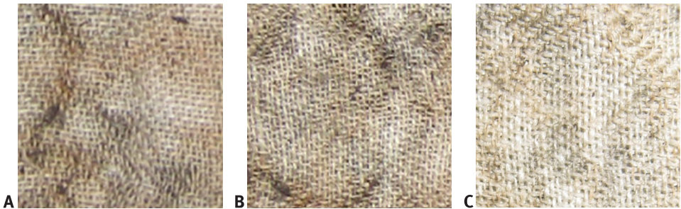
Figure 1. Visual changes of test specimens buried in soil for 4 days (29 °C, 95–100% humidity). Test specimens: A – cotton fabrics; B – unfinished specimens (cotton/linen; code T564); C – bio-textile specimens (cotton /linen with amber particles, code CL561).
