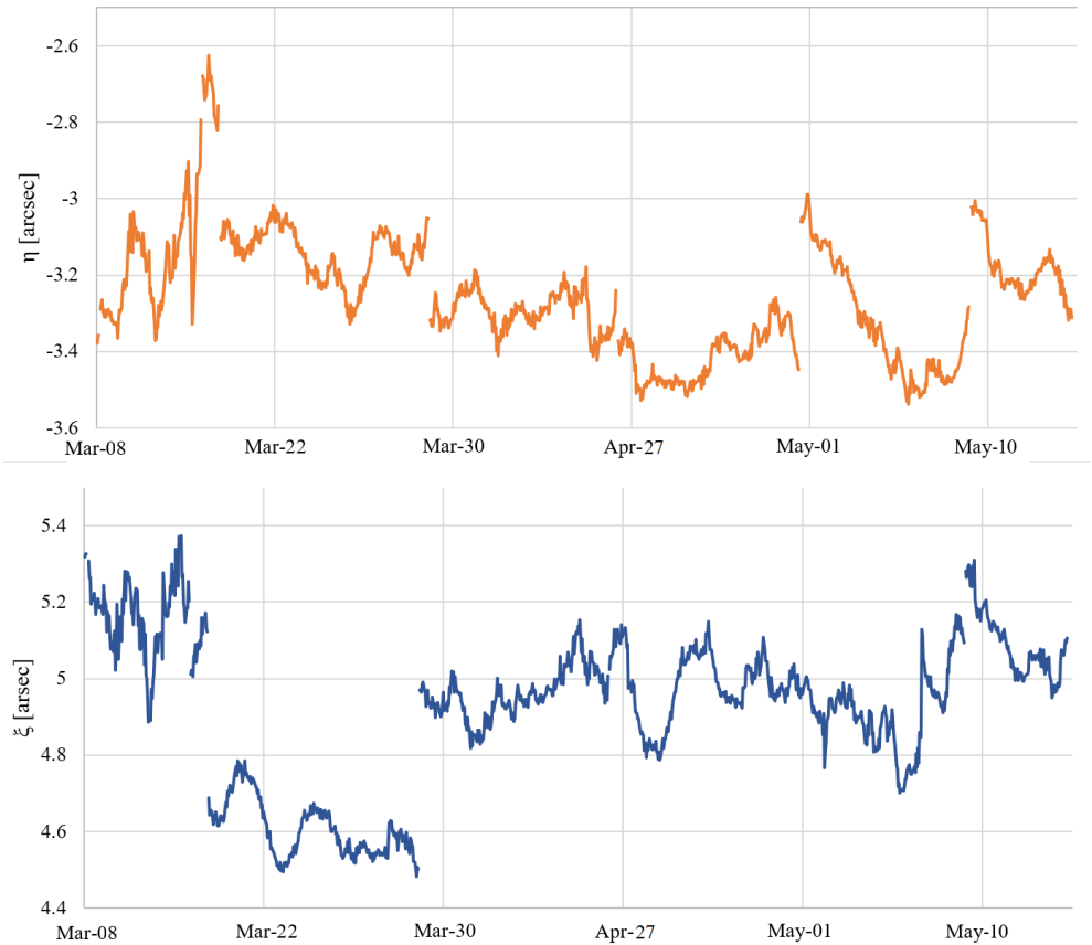
Fig. VESTA 30-position ( \sim 40 min) time window solutions of both deflection of the vertical components at Lode – multiple overnight observations during March–May 2025
