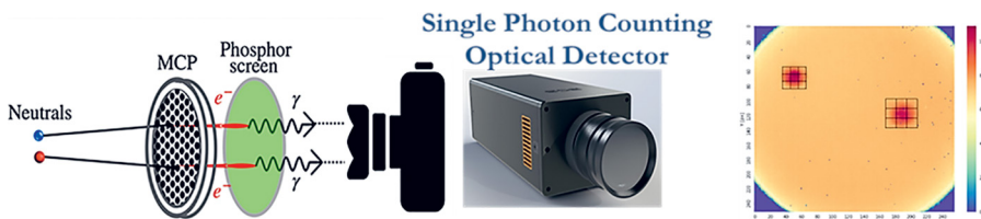
Figure 2: The MCP-phosphor TPX3CAM time-and-position sensitive detection system at DESIREE
