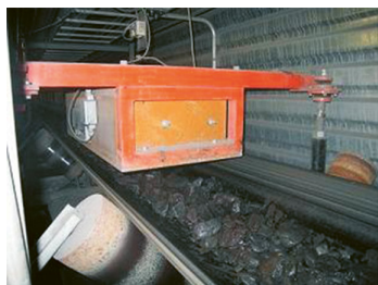
Figure 1. a) Online XRF analyser on a standard suspension on four legs above the conveyor belt of a mining enterprise; b) Spectrum of chromium-iron ore on the conveyor
